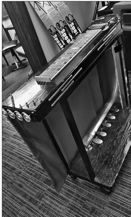
Jay Harlin’s first, four-pedal, eight-string pedal steel guitar prototype (c. 1939; a fifth pedal was added some years later); photos taken by Amy England on August 15, 2016.
